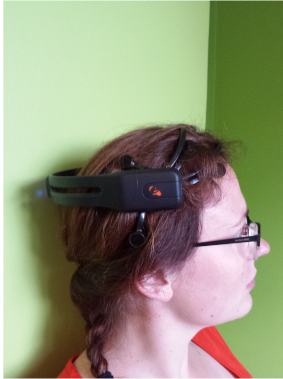
Figure 4.22: A test subject, wearing the Emotiv EPOC device during an experiment
