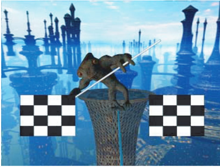
Figure 3.18: The players Avatar on a tightrope between two SSVEP checkerboards. The player must correct the avatar’s fall by focusing on the appropriate symbol [Lalor et al., 2005a]
